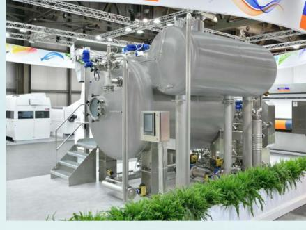
challenging dyeing tasks with ease. It excels in dyeing difficult Lycra blends of Cotton, Rayon, Nylon, and Modal fabrics in open width form, without any rope marks or edge curling.
